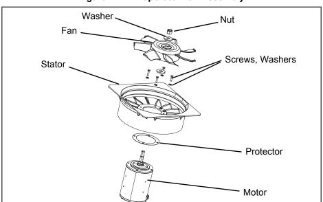
Figure 7.14 Evaporator Fan Assembly
