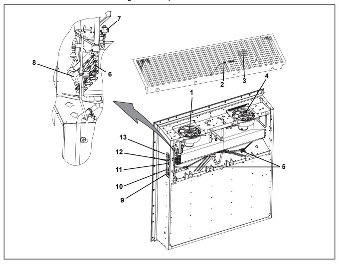
Figure 3.2 Evaporator Section
