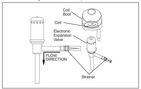
Figure 7.15 Electronic Expansion Valve
