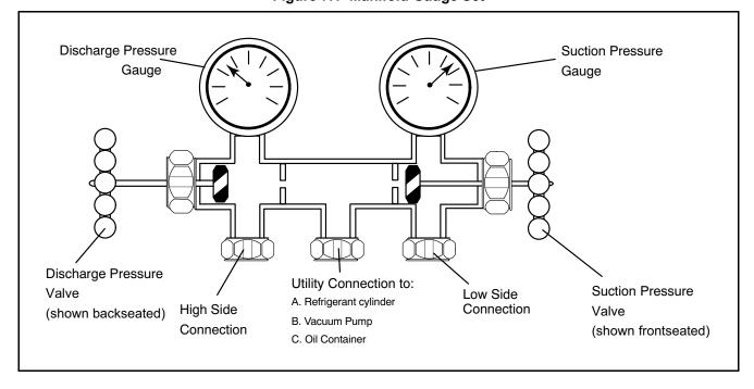
Figure 7.1 Manifold Gauge Set
