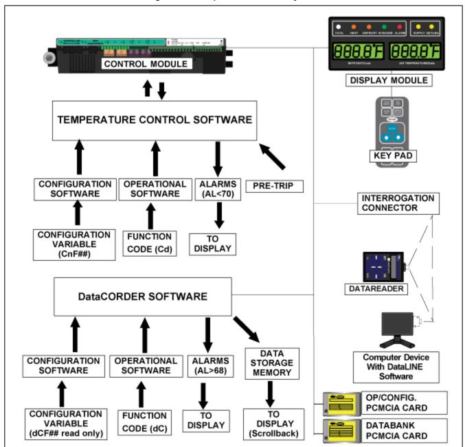
Figure 4.1 Temperature Control System
