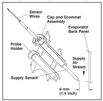
Figure 7.24 Supply Sensor Positioning
