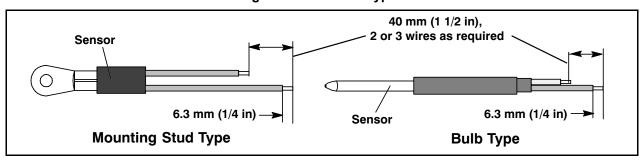
6. Slide a large piece of heat shrink tubing over the cable, and place the two small pieces of heat shrink tubing, one over each wire, before adding crimp fittings as shown in **Figure 7.23**.
