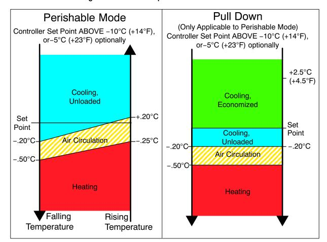
Figure 4.5 Controller Operation - Perishable Mode
