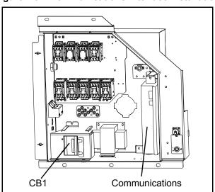
Figure 7.31 Communications Interface Installation
