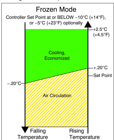
Figure 4.8 Controller Operation - Frozen Mode
