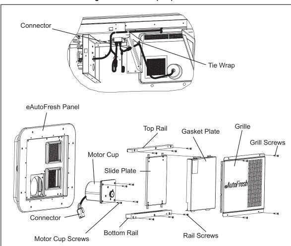
Figure 7.30 Motor Cup Replacement
