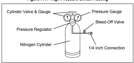
Figure 7.11 High Pressure Switch Testing
