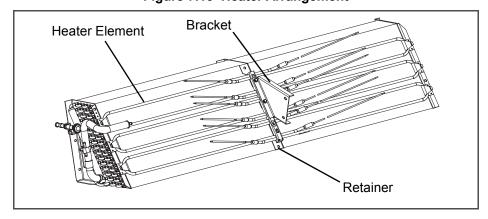
Figure 7.13 Heater Arrangement
