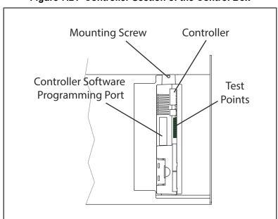
Figure 7.21 Controller Section of the Control Box
