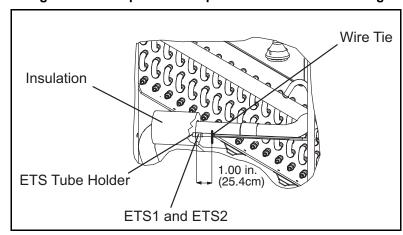
Figure 7.26 Evaporator Temperature Sensor Positioning
