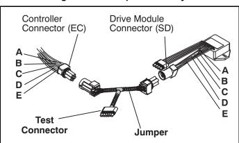
Figure 7.29 Jumper Assembly
