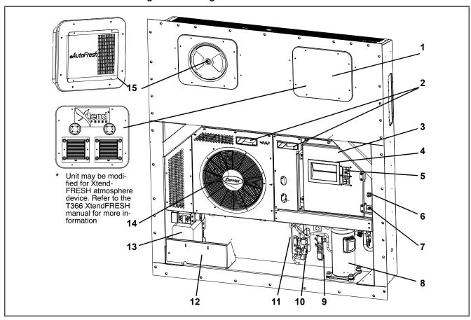
Figure 3.1 Refrigeration Unit - Front Section
