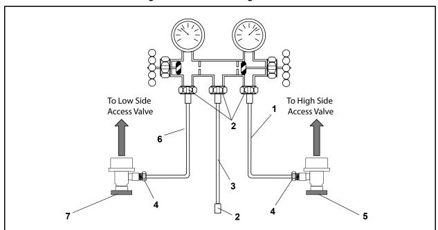
Figure 7.2 Manifold Gauge/Hose Set
