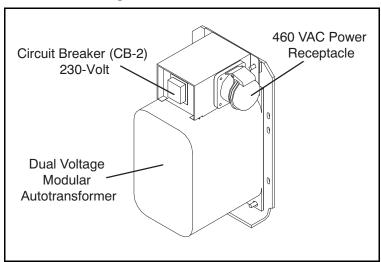
Figure 5.1 Autotransformer
